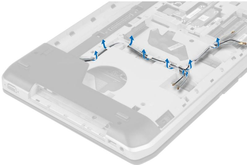
4. Desconecte o cabo LVDS (Low-Voltage Differential Signaling).
